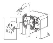
The common terminal (#4) and #3 can also be connected to a device to indicate a "full tank" state.
