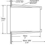
The supplied adjustable brackets allow the controller to slide into the cut-out and hold the unit in place. 95 mm (3.74") is the minimum space required to install the controller with the cables connected
