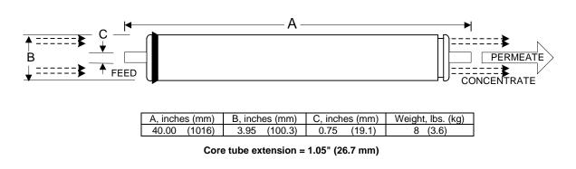
Notice: Permeate flow for individual elements may vary + 25 or - 15 percent. All membrane elements are supplied with a brine seal, interconnector, and o-rings. Elements are enclosed in a sealed polyethylene bag containing less than 1.0% sodium meta-bisulfite solution, and then packaged in a cardboard box.
